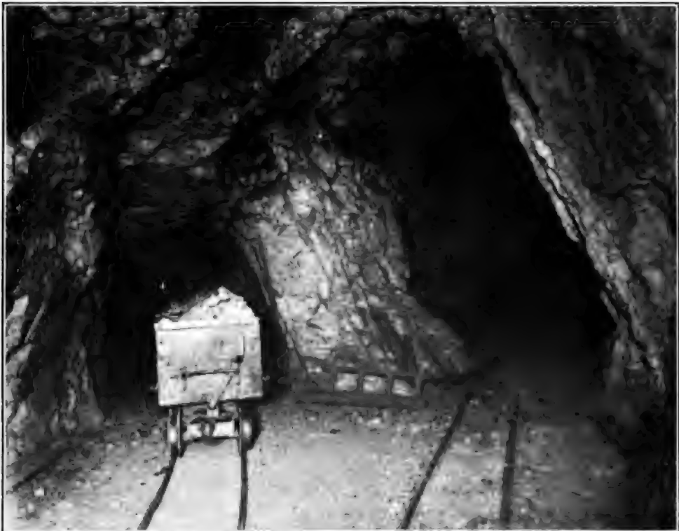
In the Humboldt mine, mules are lowered into the drifts and haul the ore to the shafts
